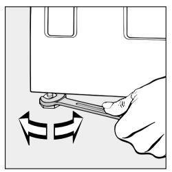
The screw feet can be adjusted to compensate for any uneveness in the floor surface. The ventilation slots beneath the door must on no account be blocked as this will prevent a sufficient intake of cold air
